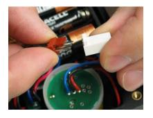
Step 8. Replace Back Cover - Do Not Pinch Wires
