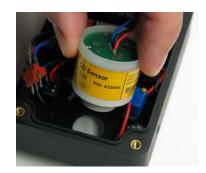
Step 7. Remove Shorting Plug from Sensor Electrical Connector & Reconnect
