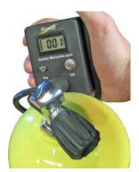
Step 4. Allow 15 Seconds for Display Reading to Stabilize
