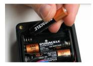
Step 4. Replace Back Cover -Do Not Pinch Wires
