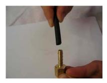
Step 2. Verify that Gas is Flowing Out Holes in Flow Adapter Cap
