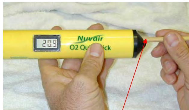
Calibrator Trim Tool Placement
