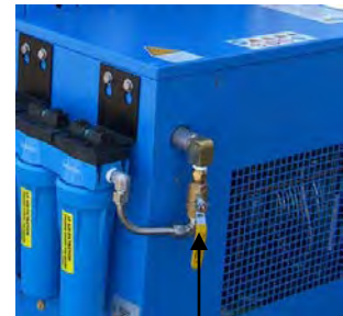
On/Off Flow Valve Handle in Off Position
