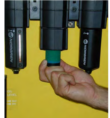
Changing LP Filtration Element
