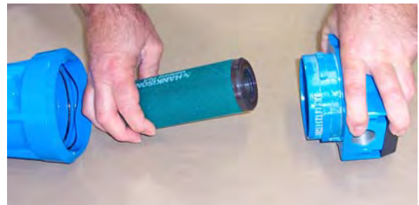
Backup Vapor Filter
