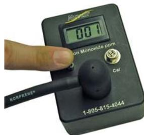
Step 3. Attach Tubing to Calibration Gas Flow of 0.5 -1 L/min
