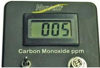
Step 6. Remove Analyzer & Verify that Gas Continues to Flow from Valve. If Not, Repeat Procedure
