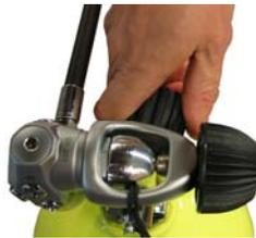
Step 3. Lightly Press Regulator Purge Button to Get Very Low Flow of Gas
