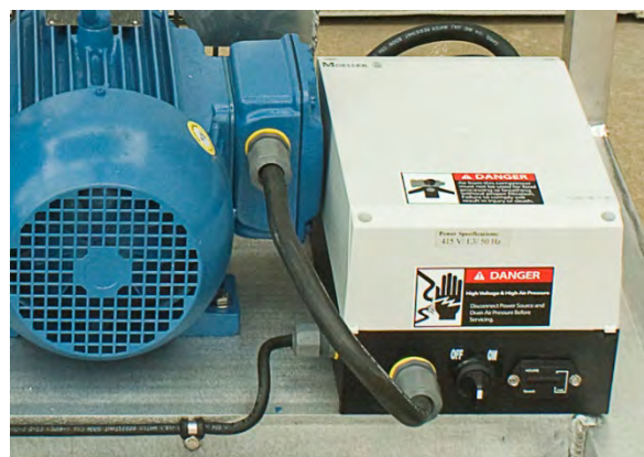
Electric Motor Power Switch and Tach.
